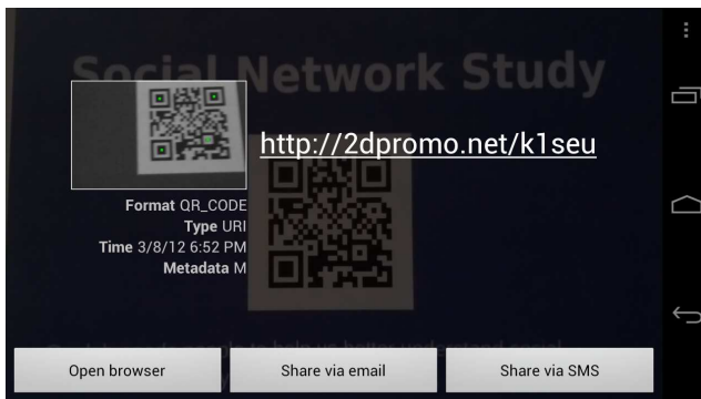
Figure 2. Screen capture of the most popular “barcode scanner” on Android: ZXing. With default settings, the URL is prominently shown to the user after scanning.
